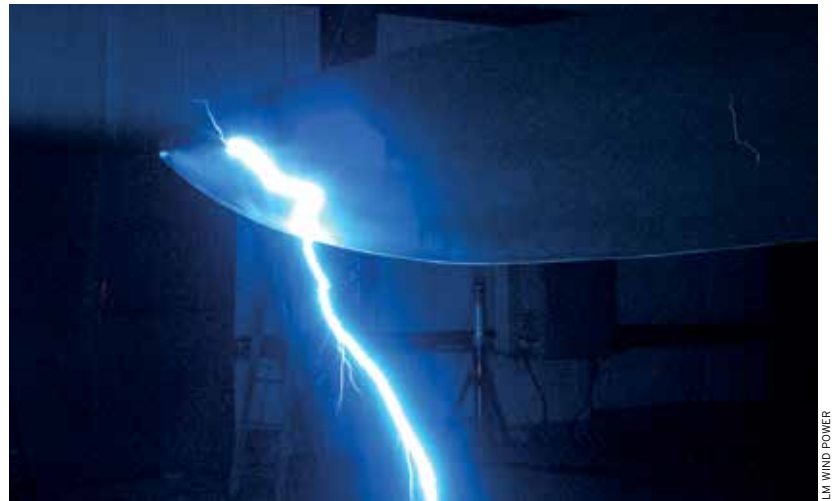
Striking Blades being tested to withstand lightning, the main cause of damage in Europe
